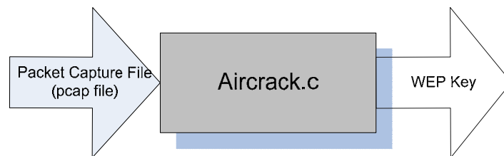
Figure 6 – Aircrack.c Input/Output Sequence
