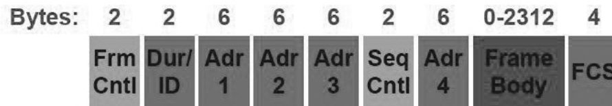
Figure 2 - Non-Encrypted Wireless Packet
